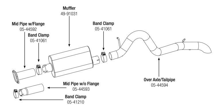
**Step 1: (Read Instructions prior to installation)** Remove your stock exhaust from the rear of your truck working your way forward. Take caution not to damage the factory isolation mounts as they will be reused. It may be helpful to lubricate the isolation mounts prior to disassembly. It is recommended to not fully tighten the clamps until the entire system has been installed.
