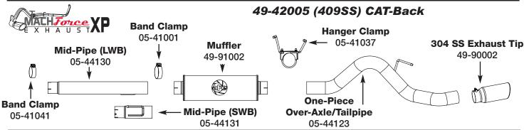
**Step 1:** (Read Instructions prior to installation) Loosen band clamp from the cat rearward. Remove your stock exhaust from the rear of your truck working your way forward. It may be necessary to cut the pipes if the slip joints are stuck. Take caution not to damage the factory isolation mounts as they will be reused.
