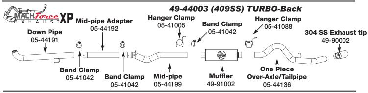
**Step 1:** (Read Instructions prior to installation) Remove your stock exhaust from the rear of your truck working your way forward. It may be necessary to cut the pipes if the slip joints are stuck. Take caution not to damage the factory isolation mounts as they will be reused. It is recommended to not fully tighten the clamps until the entire system has been installed.
