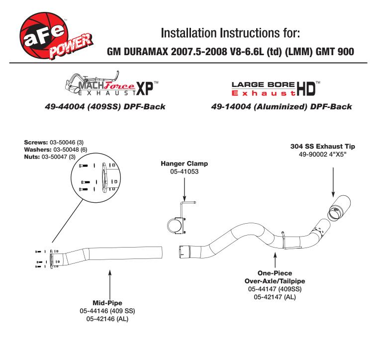
Step 1: (Read Instructions prior to installation) Loosen mounting flange at rear of particulate filter before muffler. Remove your stock exhaust from the rear of your truck working your way forward. Take caution not to damage the factory isolation mounts and gasket as they will be reused. It is recommended to not fully tighten the clamps until the entire system has been installed.
