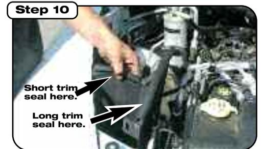
Before installing housing add trim seal. Mount shield to inner fender using OE location as seen in step 9.
