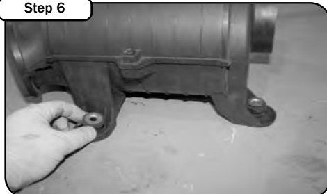
Step 6 Remove the three rubber mounts on the bottom of the airbox.Use a flathead screwdriver to remove the steel sleeve in the center.
