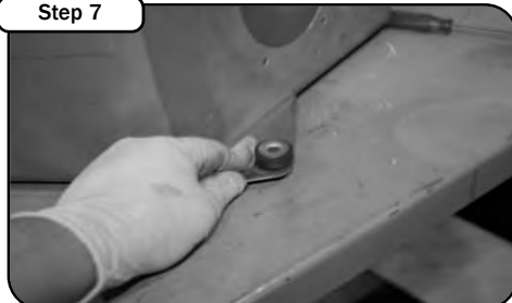
Step 7 Transfer the rubber mounts to the new air filter housing.(Hint)Use a bit if lubricant to ease installation of the mounts.
