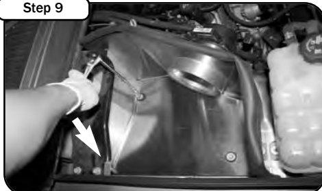
Step 9 Place the rubber trim seal along edges of the housing..Bolt the housing to the engine bay using the factor bolts removed in step 4.If installing stage 1 kit re-connect factory tube to MAF sensor.
