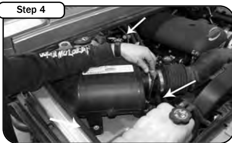
Step 4 Loosen the hose clamp connecting the MAF sensor to the filter hosing.remove the three 10mm bolts securing the housing to the engine.
