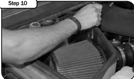
Step 10 Install intake filter into housing.Complete stage 1 system installed.Your installation is now complete .Make sure you tighten all clamps and check all electrical connections.Re check periodically.Continue onto steps 11-13 to install stage 2.
