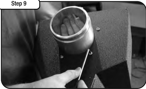
Using 4mm hex key, fasten aluminum adapter to heat shield using (4) provided M6 x 10mm button head screws.
