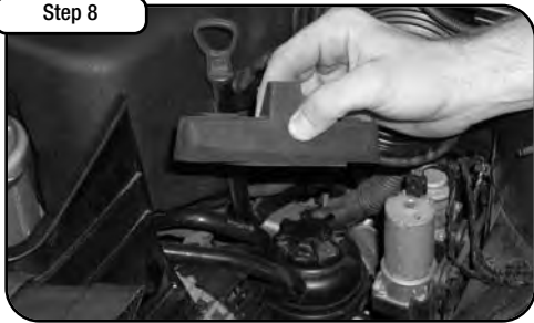
Remove rubber mount from tab beneath factory airbox.
