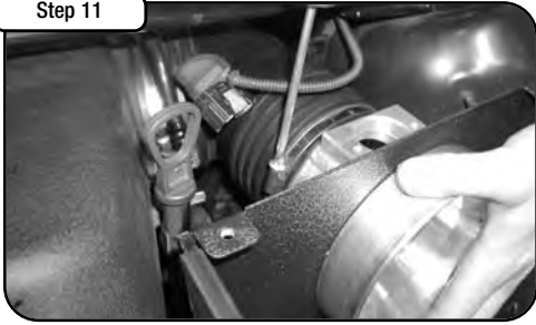
Using standard screwdriver fasten factory intake track to aluminum adapter. NOTE: it may be necessary to loosen and re-tighten the clamp securing the intake track to factory intake plenum to gain extra rotation.
