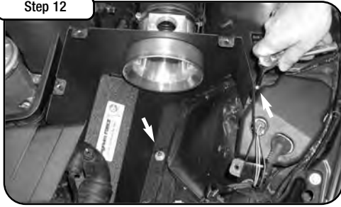
Using a 10mm socket and provided M6 nut and washer as well as original 10mm bolt, secure heat shield to engine compartment using now available mounting locations.
