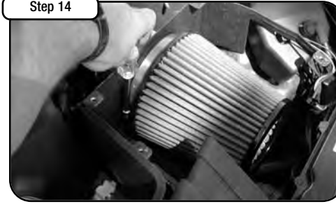
Using a 5/16" nut driver or flat blade screwdriver install pre-oiled aFe filter. Using a 4mm hex key install (4) M6 x 12mm button head screws
