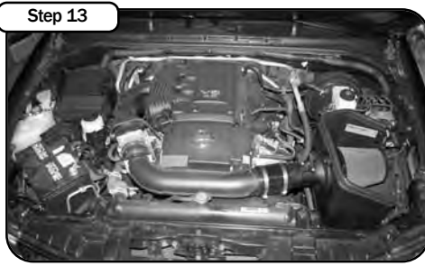
Step 13 Your installation is now complete. Make sure you tighten all clamps and check all electrical connections. Re check periodically
