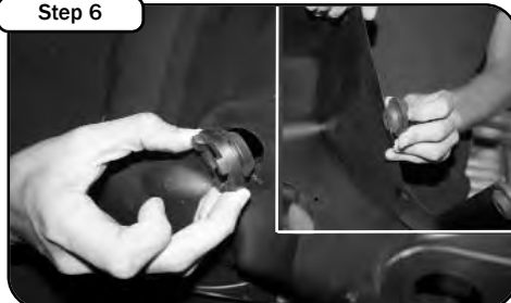
Step 6 Transfer the rubber vibration mounts located on the bottom of the air box over to the new housing.
