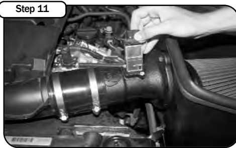
Step 11 Transfer the MAF sensor to the aFe intake tube. Secure with the supplied gaskets, spacers, and screws. Make sure you pay attention to the direction of the arrow on the MAF sensor.
