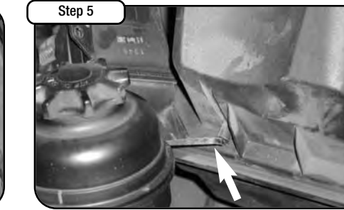
Detach resonator box from stock air box assembly using 8mm socket.
