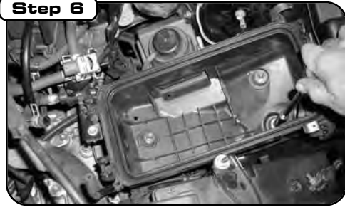
With sensors disconnected, now remove upper airbox portion. With upper airbox removed, loosen and remove bolts holding lower airbox. Loosen and remove bolt holding lower VSV mount to lower airbox (indicated by arrow). Now remove lower airbox.
