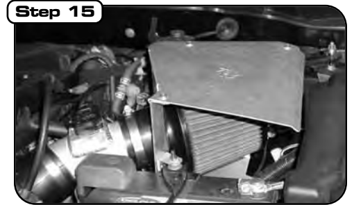
Install heat shield lid. Securely tighten all connections and re-check as necessary.
