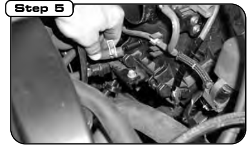
With intake tube now removed, there is a 3/8" vacuum line connected to lower portion of airbox and leading the lower VSV. Disconnect this line from the lower airbox.
