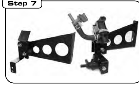
Using provided hardware, install VSV mounting tab to bracket. The rubber isolators will use (1) wavy washer per threaded side. NOTE: Be sure to mount tab with proper orientation as shown in picture.
