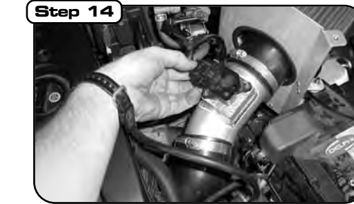
Remove the MAS from the factory airbox and re-install on aFe intake tube using provided hardware. Reconnect factory wiring harness to the MAS.
