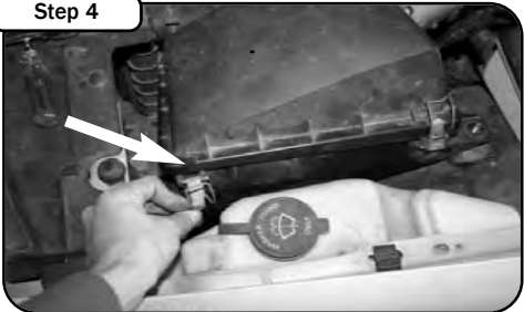
Unclamp the 2 factory airbox clips.
