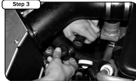
Step 3 Remove the vent tube connector from the air injection hose.
