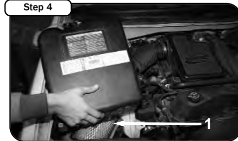
Step 4 Remove the air box housing. (1) Remove the stock air filter.
