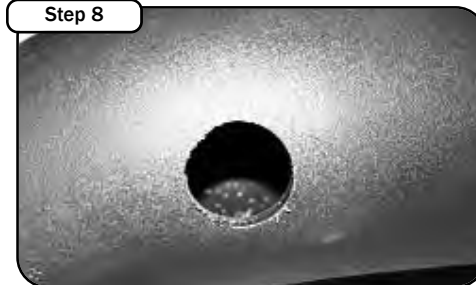
Step 8 Remove the debris from the intake tube.
