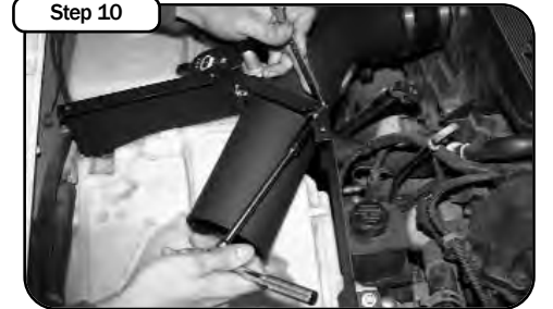
Step 10 Next using the 2 longer screws, 2 washers each, wavy washer and bolts. Fasten the housing onto the intake tube.
