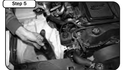
Step 5 Remove the air tube.
