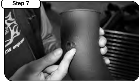
Step 7 Insert the "air temp. sensor grommet" into the aFe intake tube
