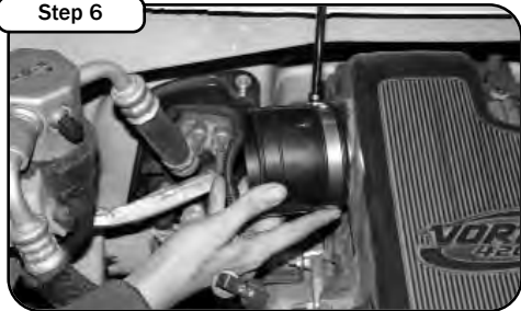
Step 6 Slip the coupler over the intake manifold and secure with a clamp.
