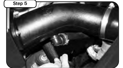
Step 5 Position the elbow so it sits inline under the intake tube. Mark the center of the location.
