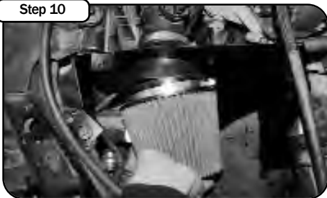
Install aFe filter onto 3-angle adaptor.
