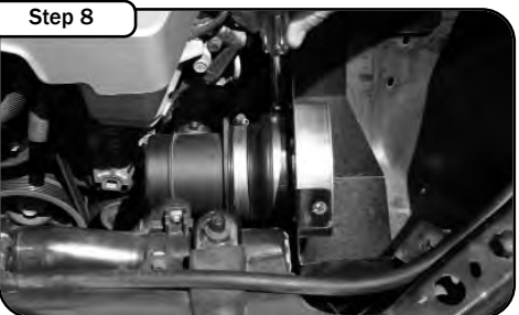
Install mass sensor and reducer coupler onto 3-angle adaptor.
