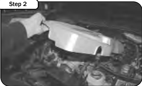
Remove oil cap, then pull up on engine cover to release from its retainers.
