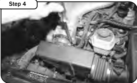
Loosen the two hose clamps from the intake plenum. Remove plenum from vehicle.
