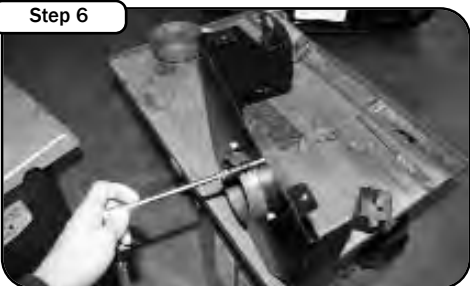
Install provided 3-angle adaptor onto aFe housing using supplied M6 hardware.
