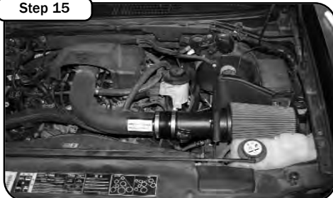
Your installation is now complete. Close hood slowly to verify hood clearance. Check and retighten connections and filter after a few hours of operation.
