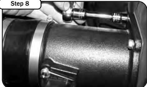
Mount the MAF sensor tube using the supplied gasket to the outside of the air filter housing, use injection molded adapter on filter side. Use the (4) M6x1x20 screws and tighten down with a 10mm wrench.
