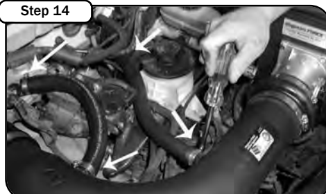
Install the 3/4" idle air bypass hose and the 5/8" breather hose on the intake tube and tighten down clamps. If you do not have a idle air bypass valve seal with the provided 3/4" vacuum cap. Install air filter and tighten the clamp.
