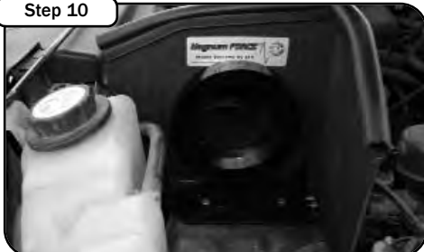
Insert the air filter housing into the engine bay and bolt down the housing to the bottom bracket with the supplied nuts and bolts. Reinstall the 8mm bolt that secures the cruise control.
