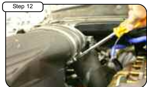
Step 12 Tighten clamps at upper-cover with 5/16" nut driver.
