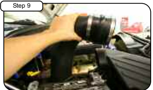
Step 9 Install hi-temp & hump coupler with clamps provided to tube. Now install tube into vehicle. Do not tighten!
