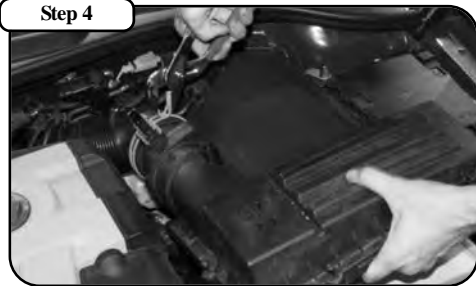
With a pair of pliers, loosen the clamp holding the tube to the MAF sensor to the stock intake tube and remove the cover and sensor from the vehicle.
