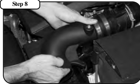
Insert the aFe intake tube along with the coupling and clamps onto the MAF sensor. Secure the intake tube using the provides screws.
