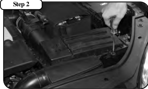
Remove the (8) screws holding the stock cover to the housing.
