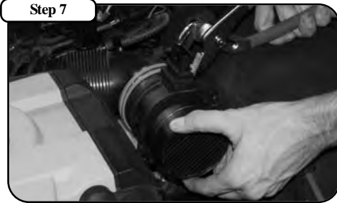
Re-insert the MAF sensor into the stock intake tube.
