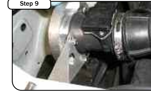
Step 9 Position the intake assembly on to the support bracket and mount the assembly with the M6 screws.
