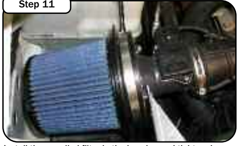
Step 11 Install the pre-oiled filter in the housing and tighten down clamp. DO-NOT use any oil or grease. Install the housing trim seal on the sides of the panel.
