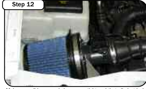
Step 12 Make sure all hoses and clamps are tight and that all electrical components are secure. Re-check after a few hours of operation. Place the included CARB EO Sticker on or near the device on a smooth, clean surface. E.O. identification label is required in passing the Smog Check Inspection.
