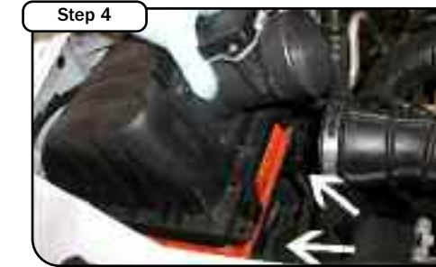
Step 4 Depress the two mounting tabs located on the side of the airbox. Lift the top half of the airbox out and remove..
