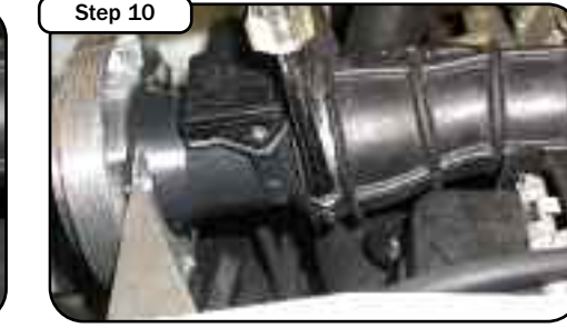
Step 10 Reconnect the MAf sensor and tighten down the hose clamp.
