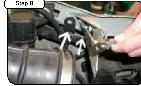
Step 8 Mount the air filter support bracket on the inside of the radiator core support. There is existing screw that support the wiring harness and a open hole next to it. Use the factory screw and the supplied M6 screw and nut. (If your truck does not have this extra hole you will need to drill a 1/4" hole in this location)
