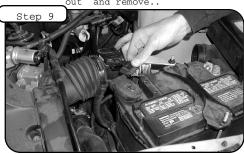
Install the pre-oiled filter in the housing and to down clamp. DO-NOT use any oil or grease.
