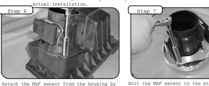
Bolt the MAF sensor to the billet adaptor using Remove the 10mm bolt supporting the battery the supplied M6 screws and washers.On the right strap.Position the intake assembly into the engine side of the sensor place the aluminum bracket bay. Line up the hole on the bracket with the battery and fasten to assembly as shown in photo.
