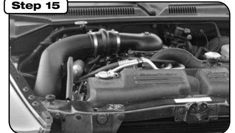
Make sure all hoses and clamps are tight and that all electrical components are secure. Check and retighten connections and filter after a few hours of operation.
