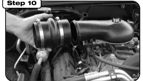
Install hump coupler to throttle body cap. Tighten clamp at cap side only.
