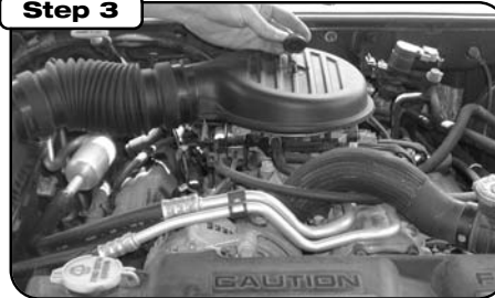
Remove nut from top of OE throttle body cap.
