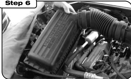
Pull out OE intake system.
