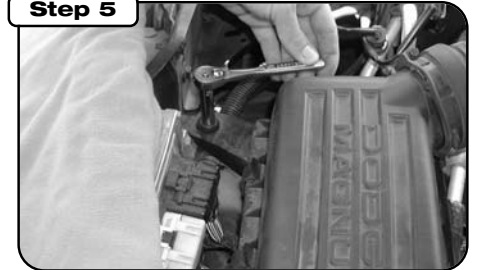
Loosen and remove bolt (one only) from OE filter box.
