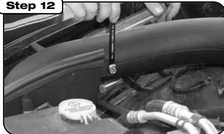
Before tightening hose clamp on coupler attach intake tube to filter housing by means of 1/4 x 20 bolt and rubber washers, flat washers and lock washer. A steel/rubber washer should go on each side of metal housing tab.
