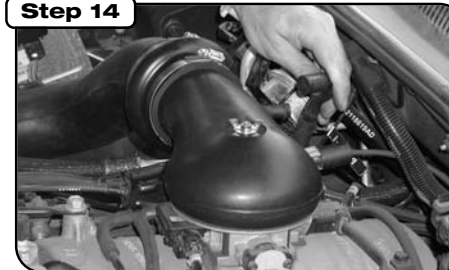
Slip vent breather hose onto cap nipple.
