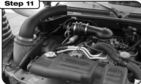
With filter attached to intake tube slide complete assembly filter first into filter housing, then slip intake tube into hump coupler.
