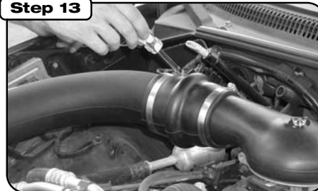
Tighten clamp at intake tube side of hump coupler. DO NOT OVER TIGHTEN.
