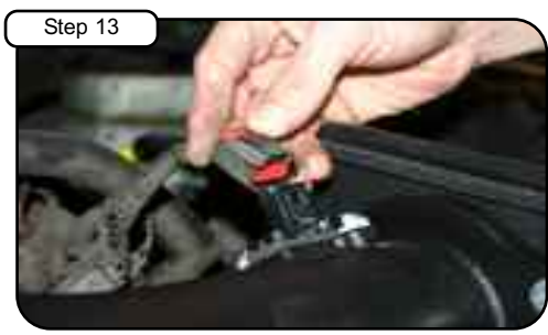
Reconnect MAF sensor harness.
