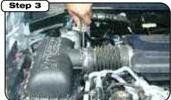
Remove air box inlet tube.
