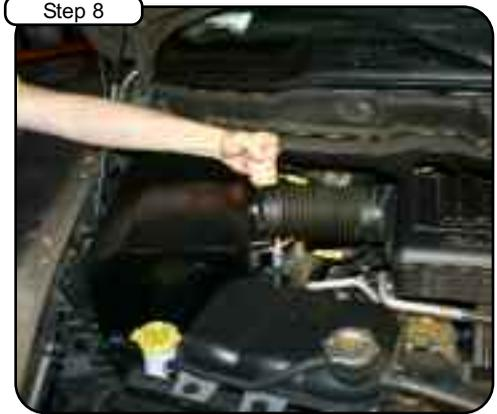
Re-connect air duct to the air filter housing. Tighten the factory hose clamp.
