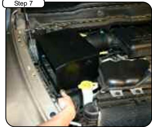
Insert housing assembly into the lower portion of the factory airbox. Secure housing with the factory airbox clips.
