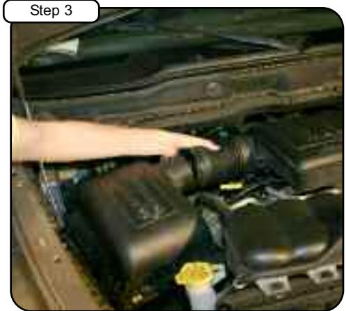
Loosen hose clamp on the air duct connecting to the airbox. Disconnect the breather hose (if equipped). Move air duct to the side
