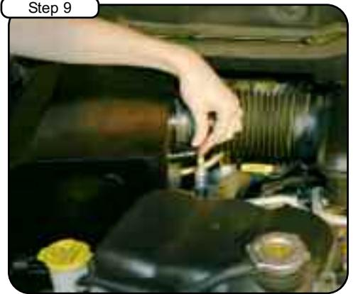
Re-connect your breather hose to the filter nipple. If your vehicle is not equipped with a breather hose, cap off the nipple with the supplied vacuum cap.
