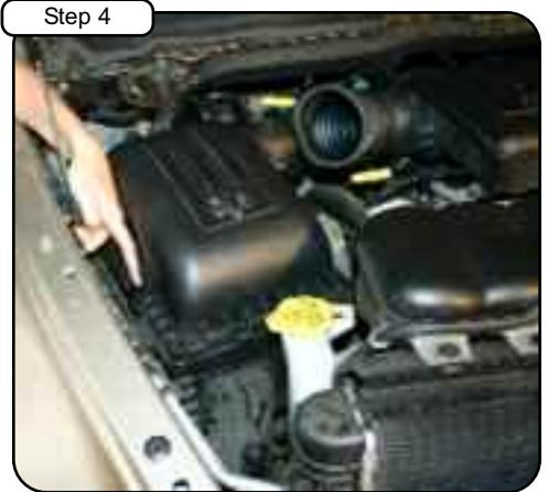
Loosen the four clips securing the upper portion of the airbox.
