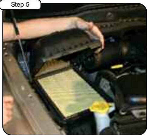
Remove upper portion of the airbox. Lift up and remove the factory paper filter.
