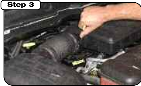
Loosen clamp at resonator box.
