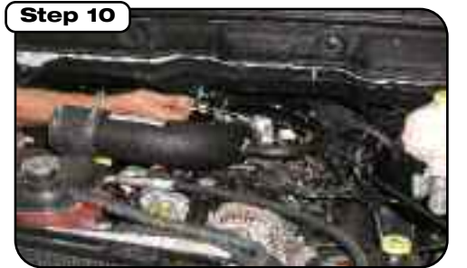
Place Intake tube "L" Bend in place. Tighten hose clamp and connect temperature sensor if applicable.
