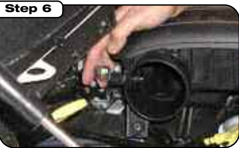
Remove temperature sensor wire harness and vent hose from resonator box.
