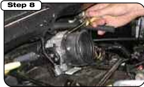
Remove stock resonator boot.
