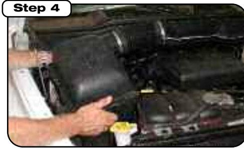
Pull off boot from resonator box and remove complete filter box assembly.
