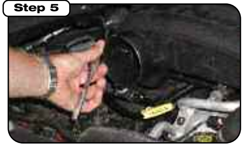
Remove the two resonator hold down bolts.
