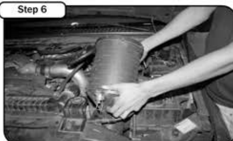
Remove the inlet portion of the air box out of the engine bay.
