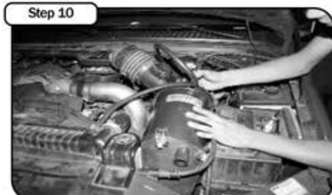
Carefully install the air box outlet, make sure the tangs engage on the bottom of the air box. Check to make sure the clamps are tight.
