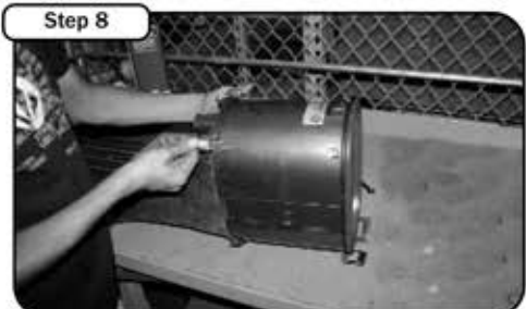
Transfer the inlet portion of the air box to the new aFe air box and secure with the factory clips.
