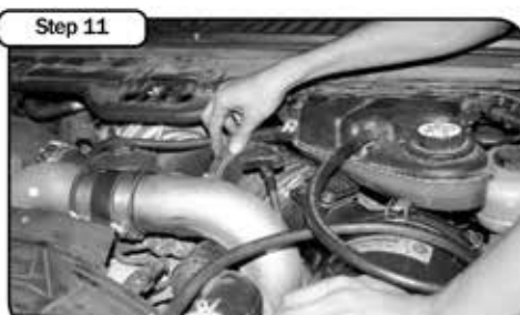
Tighten the clamp on the turbo inlet. Reconnect the MAF sensor wiring harness and the filter minder harness.
