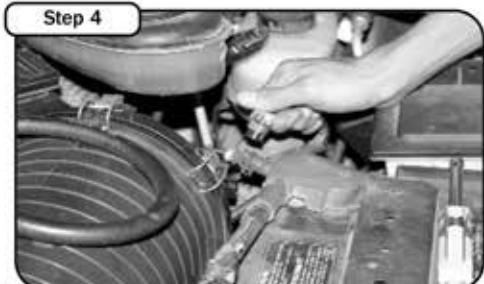
Disconnect the Filter Minder located on the back of the air filter box.
