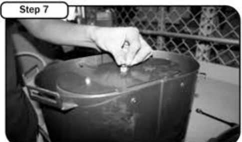
Assemble the air filter housing by placing the new air filter inside the housing, secure filter to housing with the provided nuts and washer. NOTE: The outer nut is used as a lock nut to secure filter.
