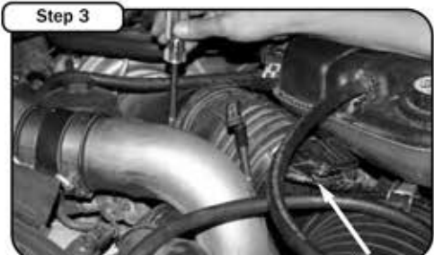
Loosen the hose clamp on the turbo inlet. Carefully disconnect the MAF sensor wiring harness.
