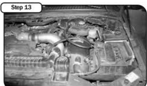
Place enclosed CARB EO sticker on a clean/smooth surface on or near the intake system. EO identification label is required in passing Smog Check inspection. Your installation is now complete. Make sure you tighten all clamps and check all electrical connections. Re check periodically.
