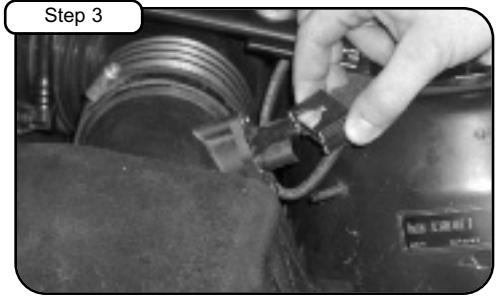
Remove factory harness from Mass Air Flow sensor and place out of the way until re-assembly.
