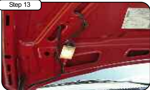
On vehicles equipped with an underhood light there may be clearance problems between the housing cover & light. The light can be removed or relocated using an existing underhood hole & screw/nut. Close hood slowly to verify hood clearance.
