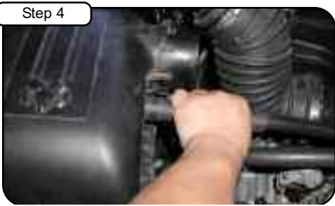
Pull out the breather hose connected to the filter housing. Then remove the factory intake duct assembly off of the engine.
