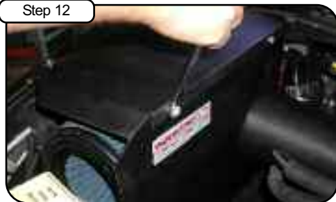
Install the cover to the housing. Fasten lid to housing with the supplied button head screws.
