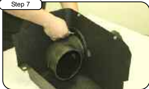
Insert the new intake tube thru the entry hole on side of the housing. Bolt the flange on the pipe to the housing using the supplied nuts and bolts. (Make sure you use the flat washer on one side and the lock washer and nut on the other side). Finally slide the urethane coupler and clamps on the end of the intake tube.
