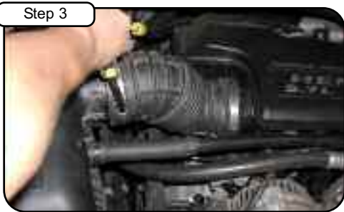
Disconnect negative post from battery terminal. Loosen the 2 hose clamps on the intake pipe.
