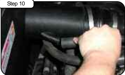
Insert the rubber breather hose into the new intake tube. The hose may have to be trimmed shorter if too long. No clamps are required. If no breather hose is used, cover vent with the provided vinyl cap.
