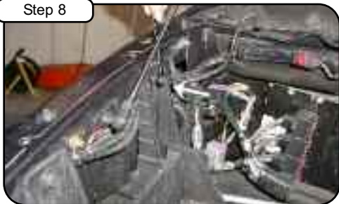
Remove the 13mm bolt on the left side of the engine bay by the hood shock. Place the assemble intake tube and housing assembly into the factory location. Line up the plastic pins on the bottom of the engine bay with the rubber grommets and lower the housing in. Line up the mounting hole on the side of the housing and reinstall the 13mm bolt.
