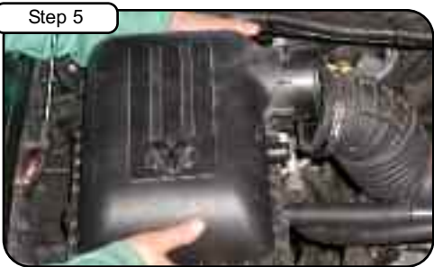
Grab the airbox from both sides and pull firmly up and out. The box is held in place with rubber grommets and lifts out very easy.
