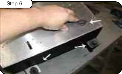
Turn over the factory airbox and remove 3 of the rubber grommets out of the box and transfer them to the new airbox in the pre-determined holes.
