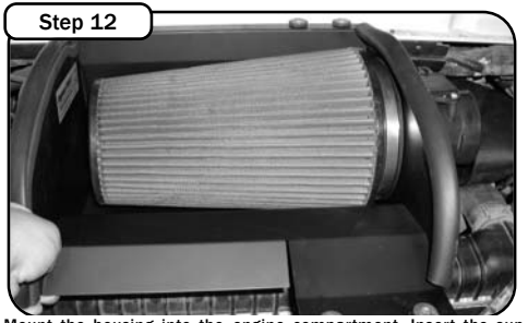
Step 12 Mount the housing into the engine compartment. Insert the supplied plastic spacer over the grounding strap location. Lower the housing in the engine bay and line up the mounting locations. Secure the housing with the (4) factory bolts. Then reinstall the bolt holding the grounding strap making sure the plastic spacer is lined up correctly. Finally tighten down all the bolts.
