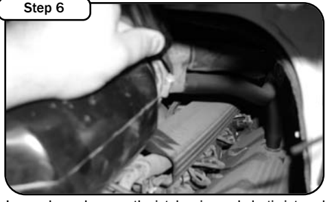
Step 6 Loosen hose clamp on the intake pipe and plastic internal baffle with a nut driver or flat head screwdriver. Remove the intake pipe and baffle out of vehicle.
