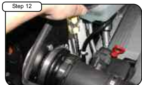
Step 12 Tighten clamps using 5/16" nut driver.
