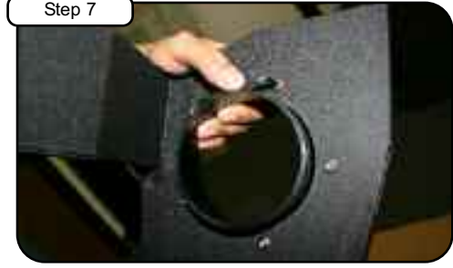
Step 7 Attach filter adaptor to inside of housing and secure using button head screws provided and tighten using 6mm allen key.
