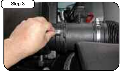
Step 3 Unclip the two silver retaining clips holding in MAF sensor.
