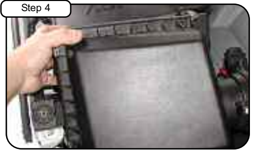
Step 4 Lift and pull out air box away from MAF sensor and remove.
