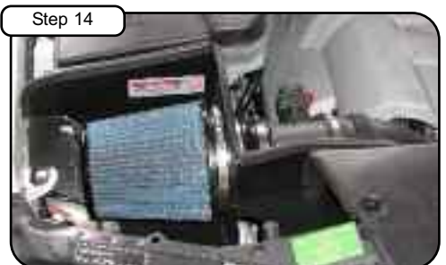
Step 14 Place enclosed CARB EO sticker on or near device on a smooth, clean surface. EO identification label is required to pass the smog inspection. Your Stage 1 installation is now complete. Make sure you tighten all clamps and check all electrical connections periodically.
