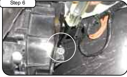
Step 6 Remove bolt from back of headlight using 5/16" nut driver. Save for later install (See step 9).
