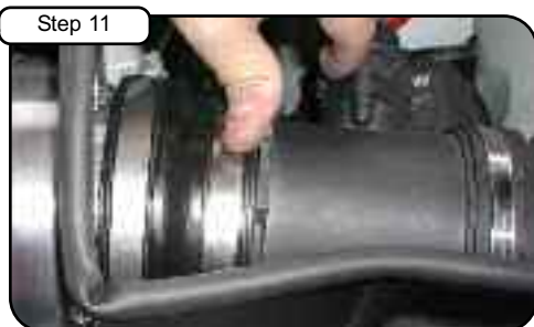
Step 11 Install reducer coupler with clamps provided to adaptor and MAF sensor.
