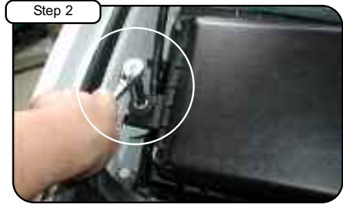
Step 2 Remove the bolt holding in air box using 10mm socket or wrench. Save for later install (See step 9).
