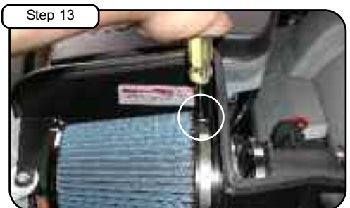
Step 13 Install air filter to adaptor and tighten using 5/16" nut driver.
