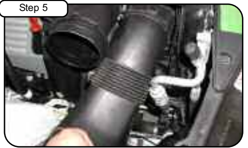
Step 5 Remove stock air duct out of vehicle.
