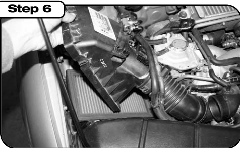
Step 6 Lift up and pull out the upper portion of the airbox and intake tube. Remove the stock air filter.
