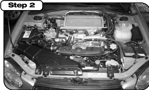
Step 2 Complete stock intake system.
