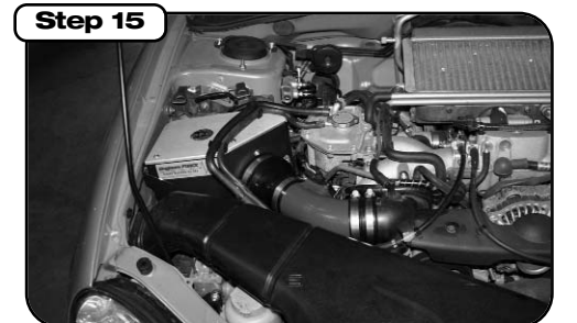
Step 15 Place enclosed CARB EO sticker on a clean/smooth surface on or near the intake system. EO identification label is required in passing the Smog Check inspection. Your installation is now complete. Make sure to tighten all clamps and check all electrical connections. Re-check periodically.
