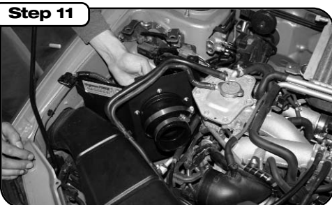
Step 11 With the housing slightly loose (for play) slip on the reducing coupler on the adaptor. *You will need this "play" to insert the aFe intake tube (tight fit).
