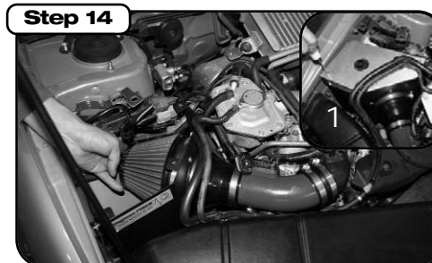
Step 14 Insert and fasten the aFe air filter. (1) Secure the housing cover with 3-M6 button head screws. Clamp the two hoses on the cover.
