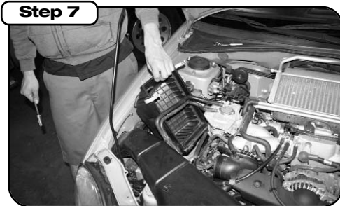
Step 7 Using your 12mm socket and ratchet extension, un-bolt the lower air box housing and remove.
