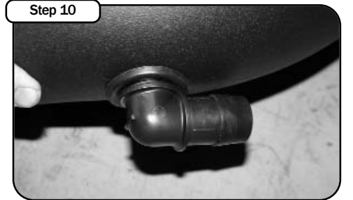
Step 10 This is a sample photo of how the elbow should be inserted into the aFe intake tube.
