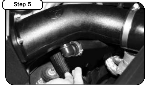
Step 5 Position the elbow so it sits inline under the intake tube. Mark the center of the location.
