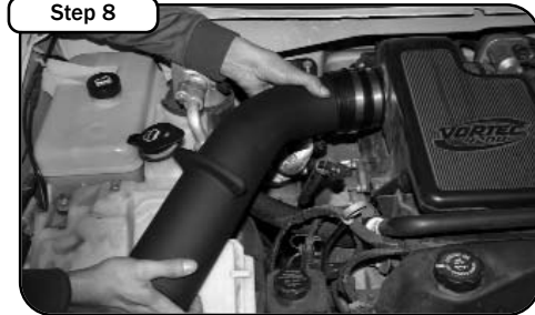
Step 8 Insert the aFe air intake tube into the coupler on the intake manifold. Once in position secure the tube using a clamp.
