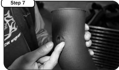
Step 7 Insert the "air temp. sensor grommet" into the aFe air intake tube
