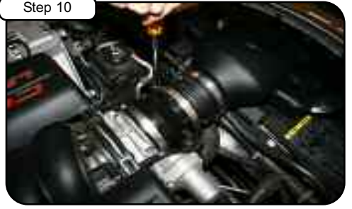
Tighten all clamps using 5/16" nut driver.
