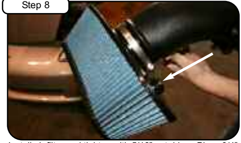
Install air filter and tighten with 5/16" nut driver. Place 3/4" cap through hole on filter.
