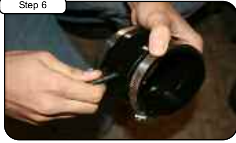
Remove OE plastic fitting from tube and install into new coupler.
