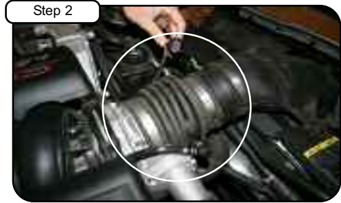
Disconnect MAF sensor harness and vacuum line. Loosen clamps with 5/16" nut driver.
