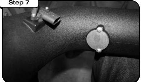
With T-20 torx bit remove temp sensor and (with gasket and screws provided) install into new tube. (5.9L place MAF cover with gasket and tighten using short phillips screws provided. Install plug into the hole in tube for crank case line)
