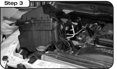
Remove factory airbox. Remove the 2 rubber mounting grommets.
