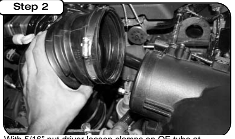
With 5/16" nut driver loosen clamps on OE tube at turbo/air box and remove. (6.7L remove crank case line with pliers and save OE plastic fitting for later install)
