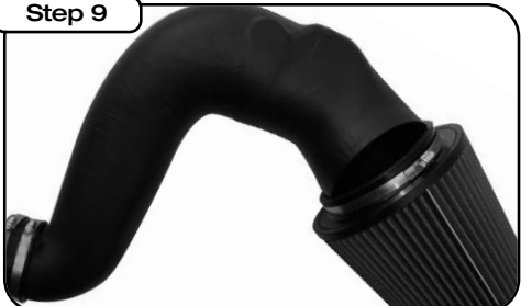
Before installing the new intake tube into the vehicle, install filter and coupler on tube ends first. Fasten the filter securely, but do not tighten coupler.
