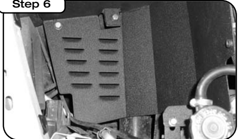
Using provided bolts, locking nuts, and washers on both sides of the bolt, fasten the intake housing. Using supplied screw and nut, fasten to housing to bracket that was installed on Step 4.
