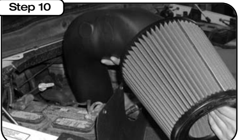
Install new tube into vehicle, slide coupler onto turbo inlet, fasten clamp assembly securely.
