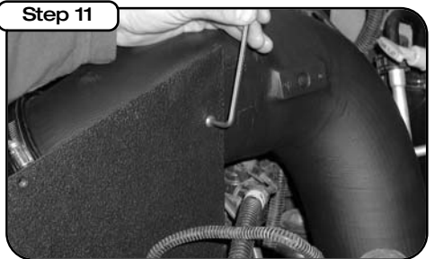
On the radiator side of the housing mount tube securely using supplied hex allen screw. Careful not to overtighten.
