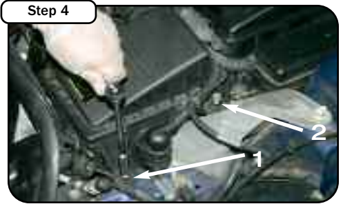
Loosen the two 10mm bolts that secure the air box on the right hand side of the engine bay. Set the bolts to the side you will be reusing these later.
