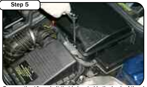
Remove the 10mm bolt that is located in the back of the air box securing the battery tray in place. Set the bolt to the side for later use.
