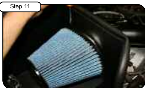
Step 11 Install air filter and tighten using 5/16" nut driver.
