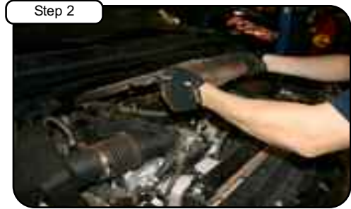
Step 2 Remove engine cover by grasping as shown and carefully lifting up.
