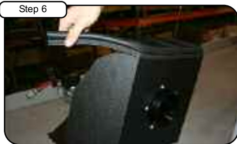
Step 6 Install filter adaptor to inside of housing using 5 button head screws and wavy washers. Tighten using 5/32 hex key. Install 3/4" trim seal to housing.
