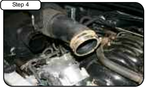
Step 4 Remove OE intake tube. Un-clip upper half of air box and remove air filter.
