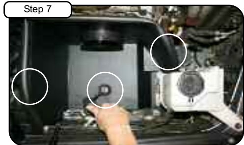
Step 7 Install housing to vehicle. Use M6 screws with flat washers provided.
