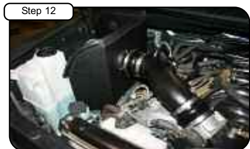
Step 12 Tighten all clamps with 5/16" nut driver. Re-connect MAF sensor harness. Re-install engine cover.
