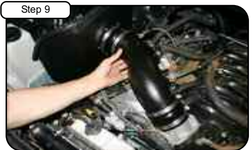
Step 9 With couplers and clamps provided install new tube into vehicle. Position tube to throttle body and housing.
