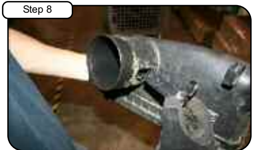
Step 8 Remove MAF sensor from stock air box.
