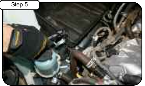
Step 5 With 12mm socket or wrench loosen the 3 bolts holding in air box. Remove complete air box out of vehicle.
