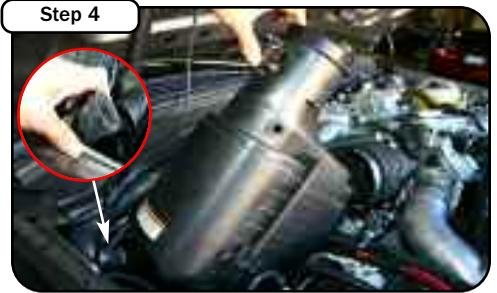
Take auxiliary air line out of air box. Lift and pull firmly then remove OE air box out of vehicle.
