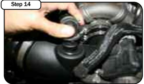
Re-install crank case line into new tube. Push down completely. Re-connect MAF sensor and filter minder.
