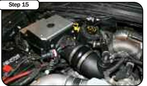
Your installation is now complete. Make sure all hoses and clamps are tight. Check and retighten connections and filter after a few hours of operation. Thank You for choosing aFe! **NOTE: Place enclosed CARB EO sticker on or near the air intake on a smooth/clean surface. EO identification label is required to pass the smog test inspection.**
