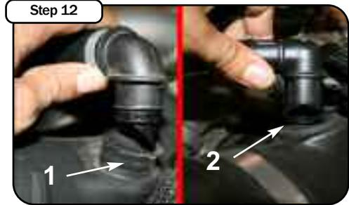
1) With cutters or pliers, cut and remove bottom OE clamp. Pull back fitting (Early production tubes which fitting can be re-used). 2) Later production tubes, cut upper clamp and use plastic fitting & mini clamp provided.
