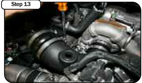
Install new tube with couplers and clamps provided. Tighten using 5/16" nut driver. Install grommet into tube.
