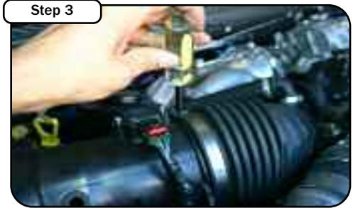
Remove filter minder out of air box. Loosen factory clamp with 5/16" nut driver. Disconnect MAF sensor harness.
