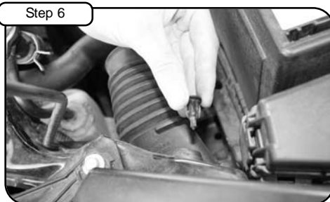
Remove small push-clip and pull out rubber air box snorkel.
