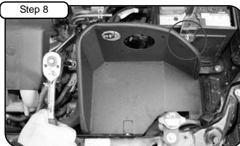
With 10mm socket or wrench, loosen battery bracket, hold tab to keep from falling and install housing. Use M6 x 1 x 20 screw and sealing washer for radiator bracket. Use flat/wavy washers and nut for isolation mount.
