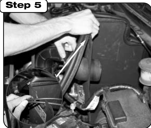
Install new housing into vehicle. Place 3-1/2" rubber edge trim in groove above Magnum Force decal. Have both cable lines between groove in housing. Now install 3/4" trim seal to housing.
