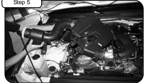
Disconnect fuel regulator line and valve cover vent line. Remove OE intake out of vehicle.
