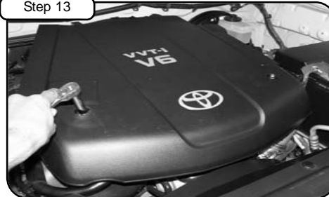
Install engine cover and use the two cover nuts from step 3 and tighten using 10mm socket.
