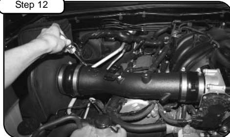
Temporarily install engine cover and position tube to align stud. NOW Tighten coupler clamps with 5/16" nut driver.
