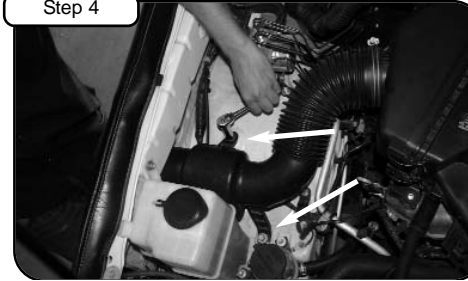
With 12mm socket, loosen the two bolts holding in OE intake snorkel. Disconnect MAF sensor harness.
