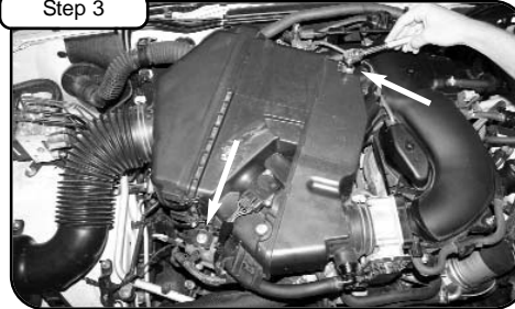
Remove engine cover with 10mm socket. With 10mm socket remove the 2 bolts holding in OE airbox. Disconnect the MAF sensor. Save the 2 cover nuts.
