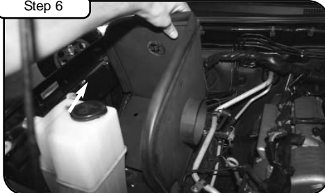
Install 3/4" trim seal to housing. Place new housing into vehicle.
