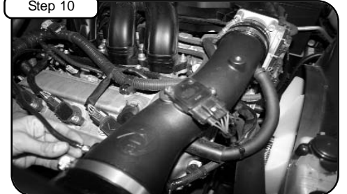
Re-connect MAF sensor harness, valve cover vent line, and fuel regulator with 5/32" hose provided.
