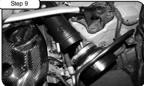
Place coupler reducer on filter adapter with clamps provided, and install tube under OE strut tower bar, keep loose to allow repositioning.
