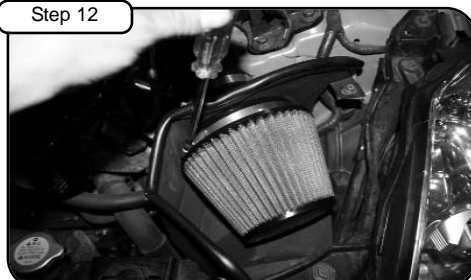
Place high FLOW filter into housing and tighten using 5/16" nut driver.
