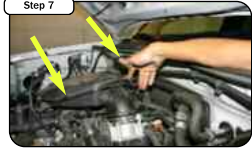
Step 7 Disconnect the breather hose and the vacuum hose connected to the intake resonator. Loosen the clamp on the throttle body. DO NOT REMOVE INTAKE RESONATOR AT THIS TIME.
