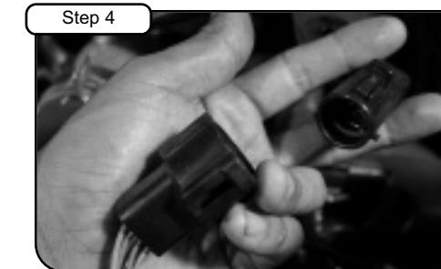
Step 4 Disconnect bottom MAF sensor harness under air box bracket.
