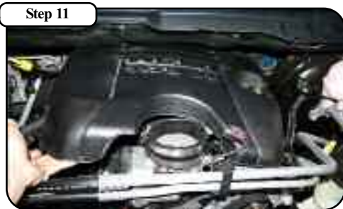
Remove the engine cover by pulling up on one side at a time to pop it loose. Install the straight coupling on the throttle body and tighten the lower clamp but leave the top clamp loose.
