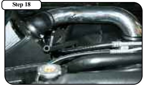
Step 18 Place intake tube into the couplings and make sure the elbow coupler is in the correct position and is not kinked before tightening all clamps.
