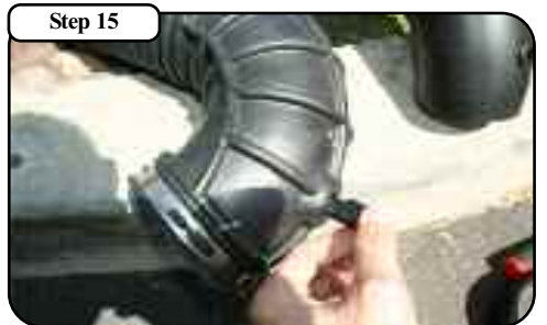
Remove the temperature sensor from the stock intake tube. Use a rag to help pull the sensor straight out. The sensor is plastic so take your time and be careful when removing.
