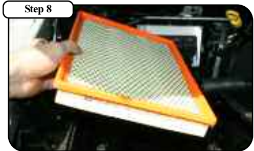
Remove the stock air filter.
