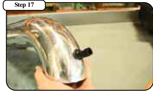
Step 17 Install your temperature sensor into the grommet.
