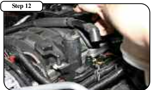
Twist the crank case breather line and pull it directly up to remove.
