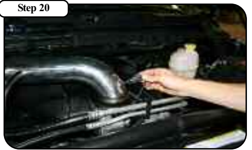
Step 20 Reinstall your temperature sensor plug and press the red tab back to lock it into position.
