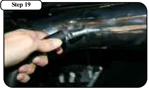
Step 19 Plug in the supplied crank case breather hose to the intake tube nipple.
