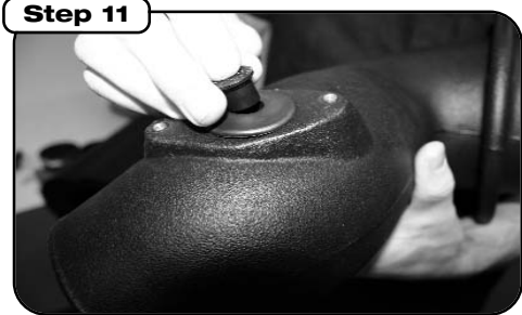
If vehicle is equipped with an air temperature sensor, use grommet in the MAF sensor opening and insert air temperature sensor into grommet. The grommet is a tight fit and may be difficult to insert.
