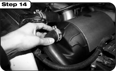
Remove factory auxiliary air tube from stock intake track and install onto aFe housing. Re-route hose under battery terminal and towards inner fender wall.
