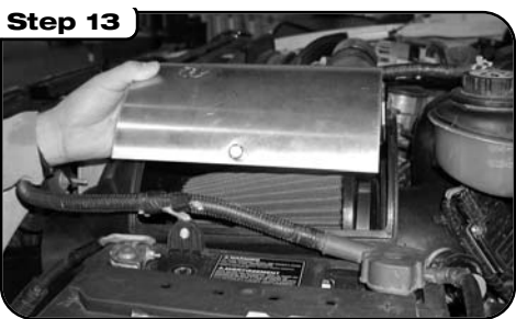
Install filter into housing and tighten clamp. Install aluminum housing lid with the aFe logo facing towards the front of the vehicle. Tighten captive screws with a snug fit.
