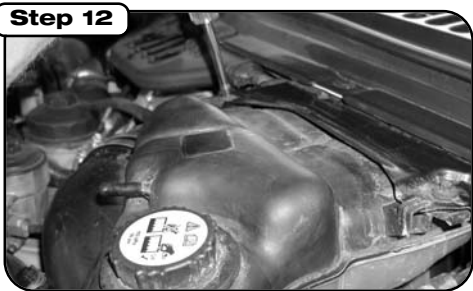
Attach tube to urethane coupler at aFe turbo inlet with provided clamp. Then use provided 1/4 20" hardware and bolt housing to tube. Reinstall radiator overflow reservoir and reconnect 1/2" hose.
