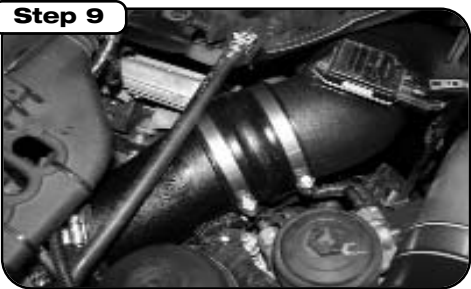
Slide tube through housing hole and turning tube to fit through. Do not attach tube to housing until Step 10. (Install MAF sensor once tube is through housing)
