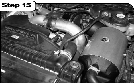
Complete intake installed. Make sure all clamps are tight and that all electrical components are secure. Check and retighten connections and filter after a few hours of operation. Reconnect battery terminal. Thank you for choosing aFe! NOTE:Retighten all connections after approximately 100-200 miles. Place the included CARB EO sticker on or near the device on a smooth, clean surface. EO identification label is required to pass the smog inspection.
