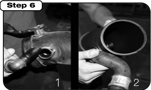
Using a 10mm socket or wrench remove tube support bracket from engine. Loosen clamp at turbo with a 5/16 nut driver or screwdriver. 1. Remove crank case breather from factory tube. 2. Place rubber grommet into with 1" opening hole and press crank case breather into grommet on new tube.
