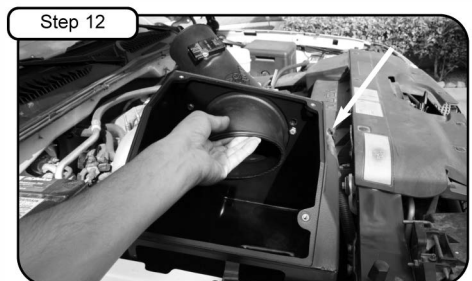
Step 12 Install housing with tube into vehicle and position.
