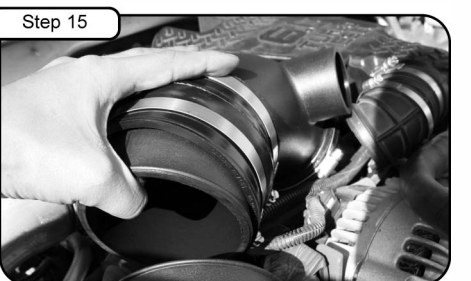
Step 15 Install tube to turbo inlet flange and position. Make sure reducer coupler is on turbo flange. Do not tighten.
