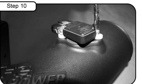
Step 10 Install MAF sensor into new tube. Use provided screws, nylon spacers and gasket and tighten using flat head screwdriver.
