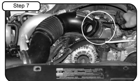
Step 7 Loosen clamp on turbo with 5/16" nut driver.
