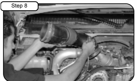
Step 8 Remove factory intake tube.
