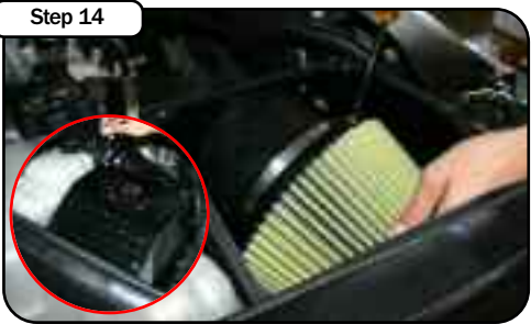
Install Air Filter and tighten using 5/16" nut driver. With button head screws provided, install housing cover and tighten using 5/32" allen key.
