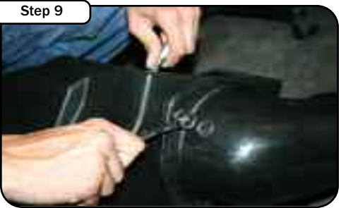
Install filter tube to outside of housing. Tighten using screws, washers and nuts provided with 7/16" socket or wrench.
