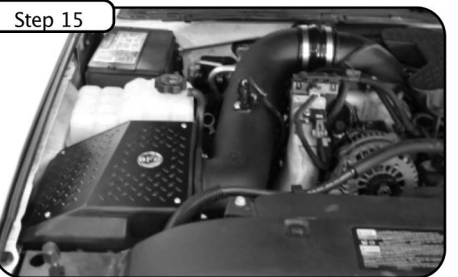
Your installation is now complete. Check all clamps and connections. Periodically check all clamps and hoses. Thank you for choosing aFe!
