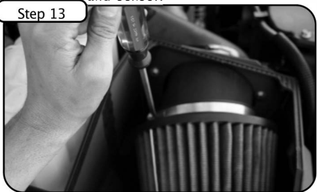
Install air filter and tighten using 5/16" nut driver.
