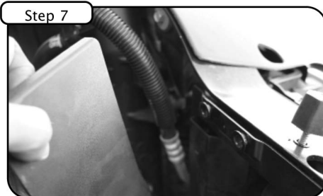
Remove plastic cover behind passenger head light.
