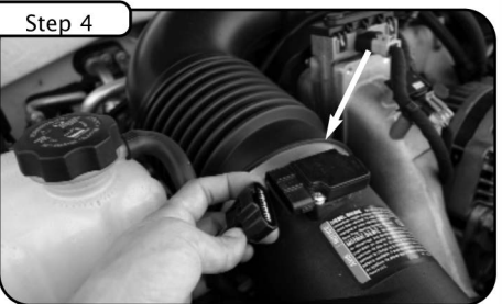
Disconnect MAF sensor harness .
