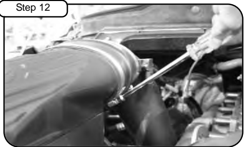
Tighten clamps at upper-cover with 5/16" nut driver.
