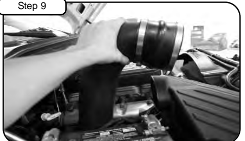
Install hi-temp & hump coupler with clamps provided to tube. Now install tube into vehicle. Do not tighten!
