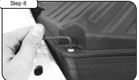
Tighten down cover housing using M6 button head screws and wavy washers.
