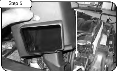
With screws provided (see step 6), install housing into vehicle. Make sure housing tab mounts up to bracket "D" from step 4.
