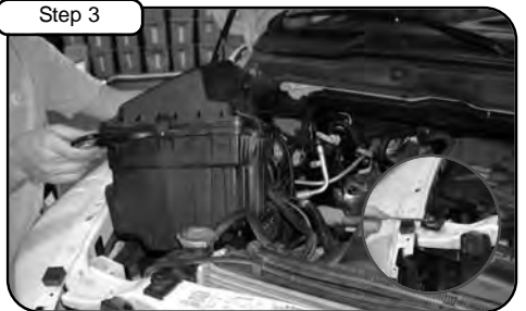
Disconnect air temp sensor. Loosen 10mm nut holding in front of air box using wrench or socket. Lift up and pull OE air box out of vehicle.
