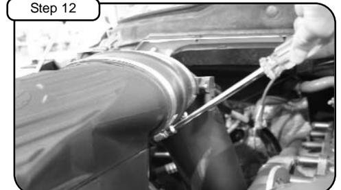
Tighten clamps at upper-cover with 5/16" nut driver.
