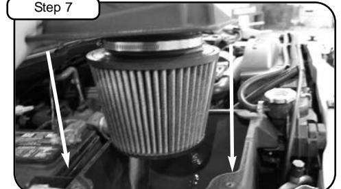
Install air filter to cover housing, tighten using 5/16" nut driver. Place cover to bottom of housing and set to position.
