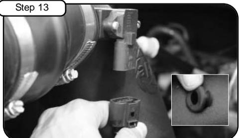
Reconnect temp sensor harness. Install filter minder grogmet in hole provided and install filter minder.
