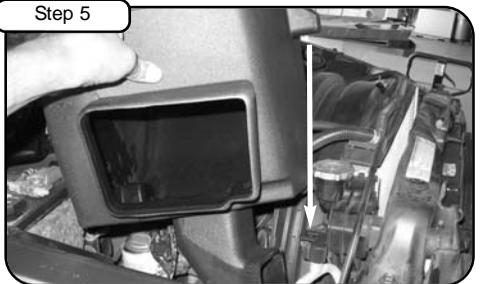
With screws provided (see step 6), install housing into vehicle. Make sure housing tab mounts up to bracket "D" from step 4.
