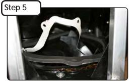
Carefully apply the sealing gasket to the air boot with the adhesive side toward the air boot. Peel the adhesive back and use the supplied bolts to help align the gasket.
