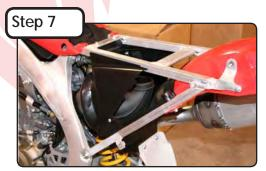
Reinstall subframe. Connect air boot to carburetor. Remember to connect the breather hose to the air boot. Tighten all bolts to factory recommended specs and use thread locker where needed.
