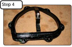
Remove filter mount and set aside. The filter mount will not be used. Clean the sealing surface of the air boot inside the airbox using alcohol or parts cleaner.
