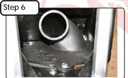
Install the intake tube, opening pointing to top of subframe. Bolt tube to airbox with washers and nuts toward front of bike. Do not over-tighten the bolts. HINT: Start with the bottom bolt.
