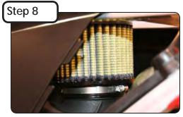
Install the inner filter onto the intake tube. First tighten the hose clamp just snug so the filter does not go past the bump on the tube. Press the filter firmly into place on the tube.
