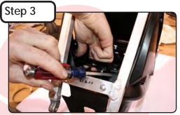
Carefully pry the filter mount away from the air box using your fingers and a large flat screwdriver. This may take some time as they are glued together.
