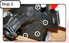
Using an 8mm socket remove the 6 nuts holding the filter mount from the front side of the airbox. Set these nuts aside, they will not be used.
