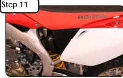
Reinstall seat and side panels. The installation of your Aries AE2 intake kit is now complete. We recommend you clean the outer filter every 4 to 6 rides and the inner filter every 12 to 18 rides depending upon conditions.
