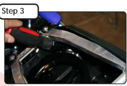
Using a 4mm allen wrench, loosen the clamp around the air boot flange.
