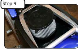
Install the outer Pro DRY S filter onto the inner filter.
