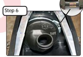
Tighten the clamp using the 4mm allen wrench. You may have to remove the spacer in the clamp to completely tighten.
