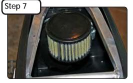
Install the inner Pro GUARD 7 filter onto the intake tube.
